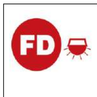
Space protected by automatic fire alarm
