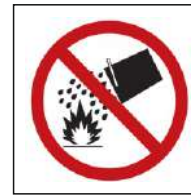
Do not extinguish with water
