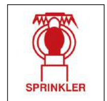
Space protected by sprinkler
