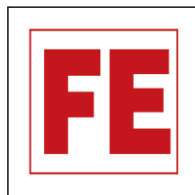
Locker with fireman's equipment
