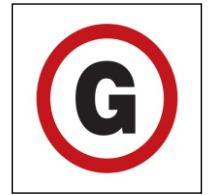
Emergency source of electrical power
