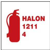
Halon 1211 fire extinguisher (4) kg
