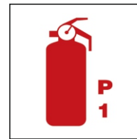
Powder fire extinguisher (1) kg
