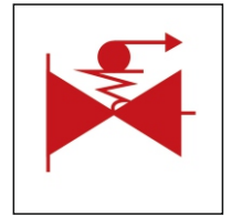
Remote controlled fuel/lubricating oil valves
